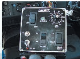
Truck Cab Panel Gives the Driver Complete Control of All Spreader Functions.
